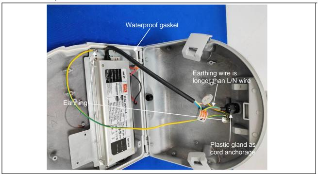
Details of: Internal view for P series models with two LED drivers Representative model: ST305P
