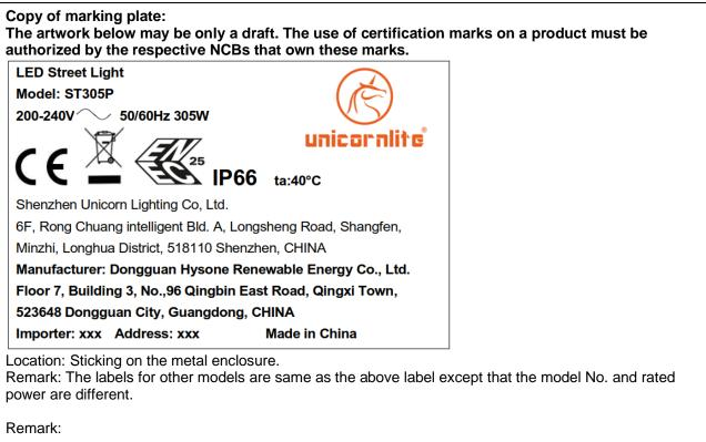
• Height of CE marking at least 5mm, height of WEEE mark at least 7mm, height of other marks at least 5mm, height of letters and numerals at least 2mm.
