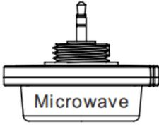
1. Microwaves cannot penetrate metal. Please avoid installing the product in a closed or semi-closed metal luminaire to ensure that there is no metal or glass shielding above the product. If the antenna must pass through the metal plate, please ensure that the top of the sensor is close to the metal plate.
